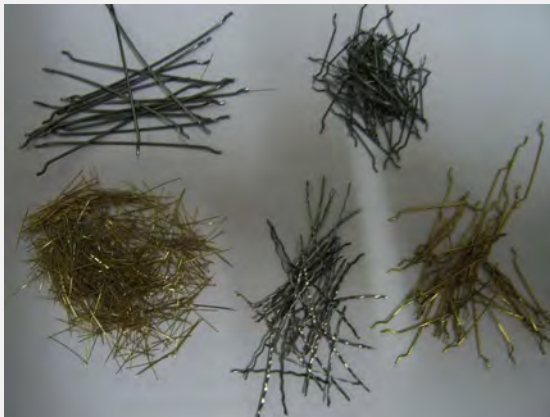
Fig 02. Types of Steel Fibers .
