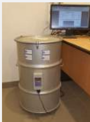
concrete calorimeter for Heat of Hydration
